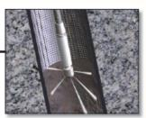
Speed controlled, high efficiency, rotational jets provide optimal well cleaning.
